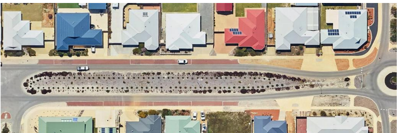
Figure 5: Crossover examples where the footpath remains continuous
